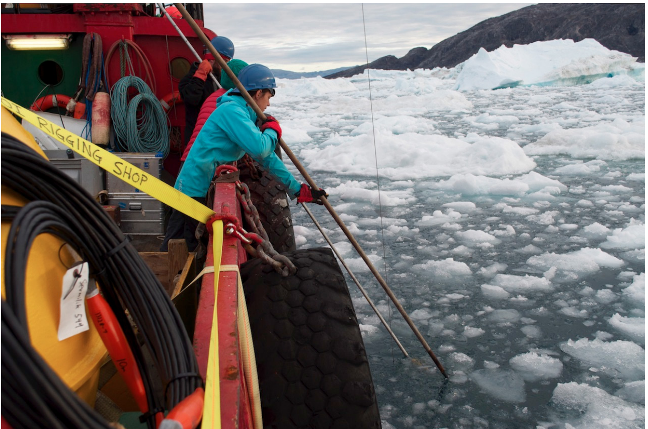
Figure 3. Researchers push ice away from a line that measures conductivity, temperature, and depth. Photo courtesy of F. Straneo.
