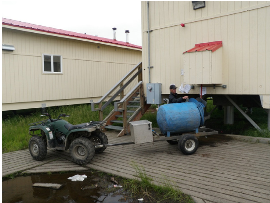
Example of a village-based small vehicle waste haul system. Photo courtesy of B. Lefferts.
