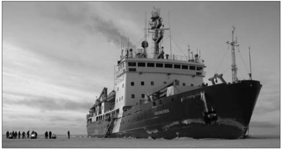
The refurbished Amundsen includes features such as an internal moon pool, providing an opening to the sea from inside the ship, fully equipped wet and dry labs, a fast-launch davit, and an acoustic well. Photo by Gérald Darnis (CASES).
