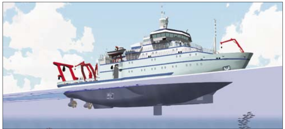
This view of the ARRV concept design shows the ice-capable hull form, retractable centerboard for transducers, and twin azimuthing propellers. Illustration by John Farmer, Farmer Marine Design Services.
