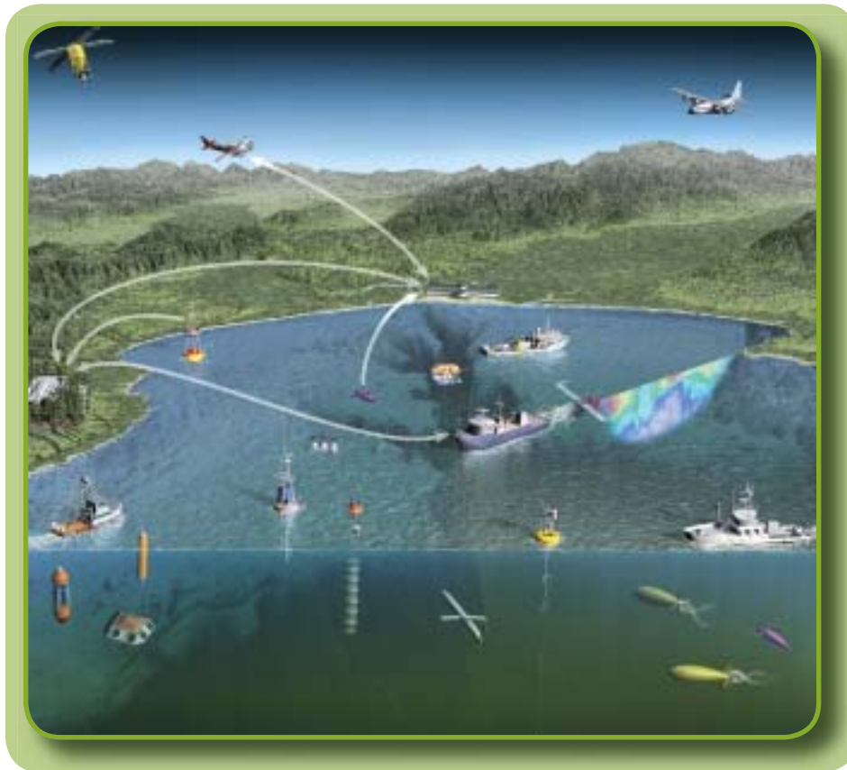
Figure 28. The Autonomous Ocean Sensing Network (AOSN) in Monterey Bay uses a variety of modern platforms to produce a comprehensive view of the ocean. An exercise during summer 2003 used gliders, AUVs, drifters, floats, satellites, ships, moorings, and aircraft. Noteworthy was the deployment of a fleet of over 20 gliders of two different designs. Data were made available within hours to computer models, which in turn provided input into decisions on continued sampling from the array of platforms. The success of AOSN is a harbinger for future regional ocean observing systems. Figure courtesy of David Fierstein, Copyright 2001, MBARI.
