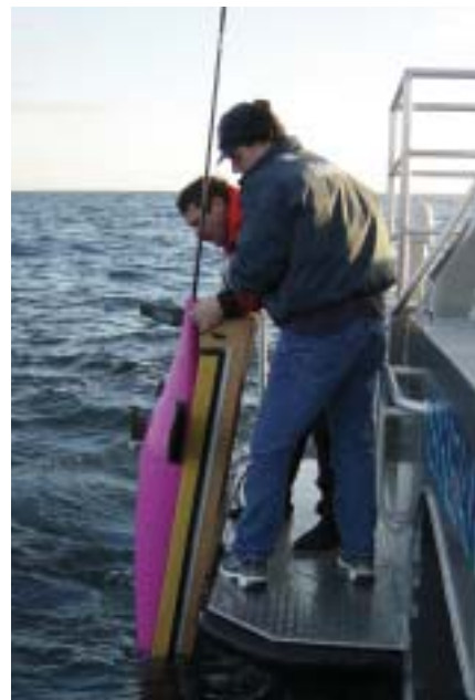
Figure 16. The Seaglider is one of several autonomous underwater vehicles that enable oceanographers to measure hydrographic, chemical, and biological fields on long sections across the oceans. This particular instrument can measure about 1000 profiles from the surface to a depth of 2 km over a track of about 6000 km. Each time it surfaces, it transmits data via satellite, at which time its course can be reset. The Seaglider is 1.8 m long and weighs 52 kg—a size and weight that allow easy launching and recovery by two people on a small boat.
