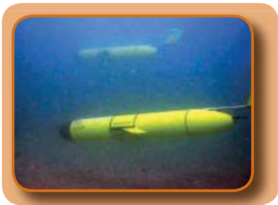
Figure 4. Two Webb Slocum gliders flying off the west coast of Florida during a red tide in January 2003. The research associated with these gliders (NSF-supported program called Operation Gulfcast) grew out of the EcoHab and ONR HyCODE programs. In the coming years, the hope is that gliders will become a routine monitoring tool for red tides in the Gulf of Mexico. See case study on p. 33 for more information. Photo courtesy of Oscar Schofield, Rutgers University.
