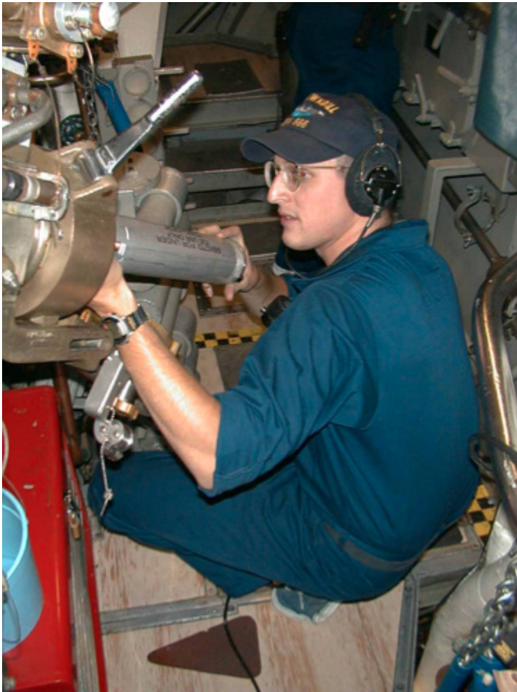
Figure 3: Navy Crewman "Ted" Groustra loads an XCTD for launching. Image courtesy of U.S. Navy Arctic Submarine Laboratory.
